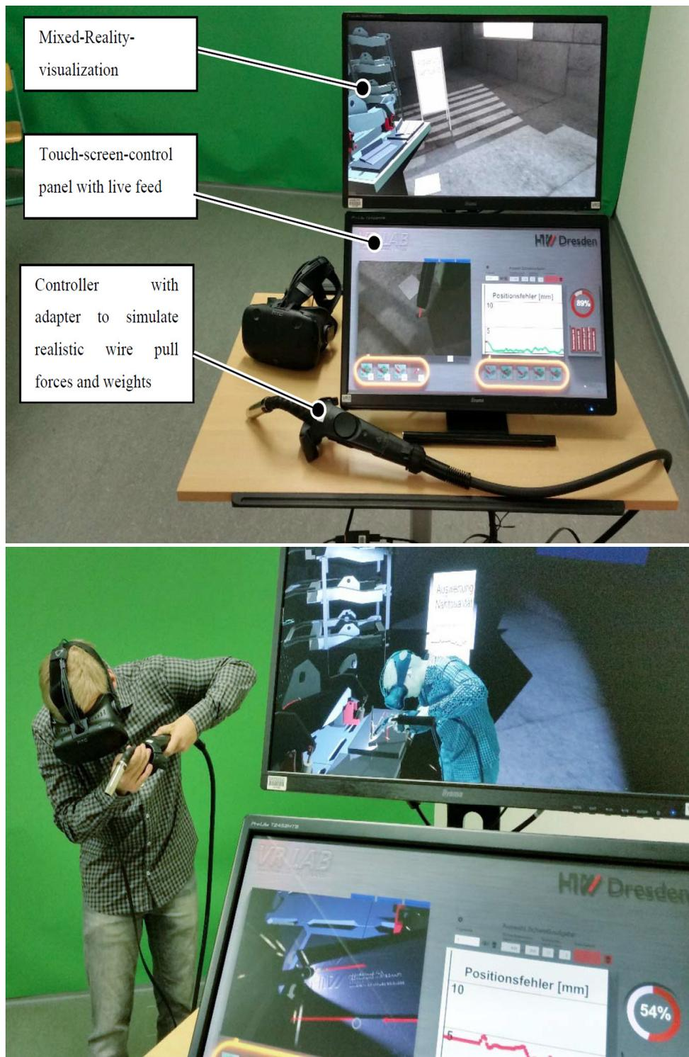
**Figure 1.** above: learning environment for manual welding (mixed reality view, control panel, head-set, controllers), below: live-impression during application
